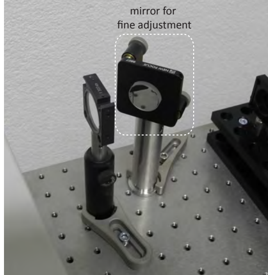
Figure 4.7: Left: During rough alignment, the green beam is positioned on top of the red beam. Right: Please use this mirror only for fine adjustment of the beams' overlap.
