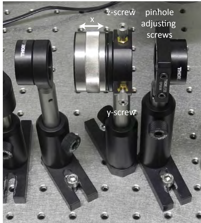
Figure 4.9: The pinhole is mounted in the silver cylinder, that can be rotated to adjust the pinhole's position along the optical path of the confocal microscope (x axis). The silver cylinder is fixed on a small yz-stage to allow for proper positioning of the pinhole in the plane perpendicular to the optical axis.
