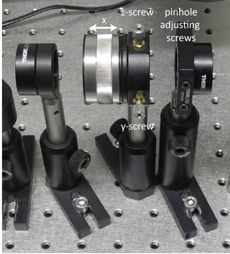
Figure 9: The pinhole is mounted in the silver cylinder, that can be rotated to adjust the pinhole's position along the optical path of the confocal microscope ( x axis). The silver cylinder is fixed on a small yz -stage to allow for proper positioning of the pinhole in the plane perpendicular to the optical axis.
