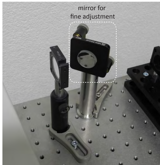
Figure 7: Left: During rough alignment, the green beam is positioned on top of the red beam. Right: Please use this mirror only for fine adjustment of the beams' overlap.
