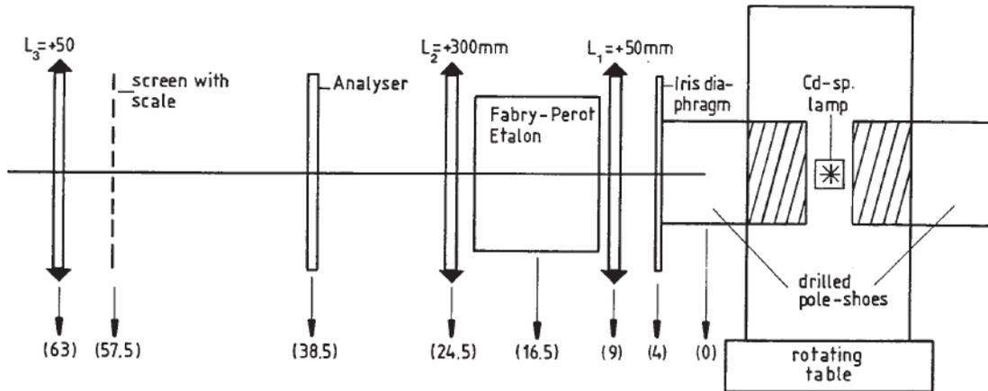
Figure 6: Scheme of the optical components
