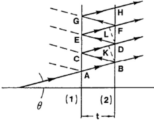
Figure 3: Transmitted and reflected rays at the étalon's parallel surfaces (1) and (2).
