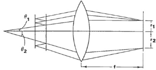
Figure 4: Focusing of the light coming from the Fabry-Pérot étalon. The light is focused onto a ring with the radius  $r = f\Theta$ , with  $\Theta$  being the incident angle of the light into the étalon and  $f$  the focal length of the lens.
