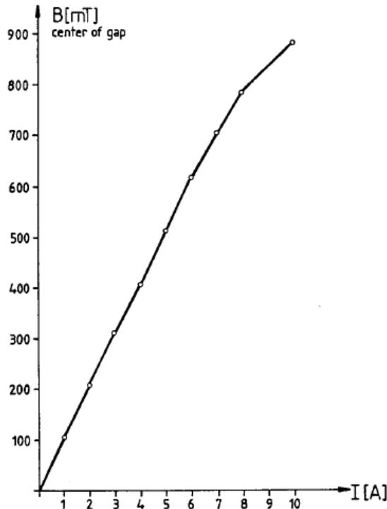
Figure 7: Magnetic flux  $B$  in between the two Helmholtz coils, where for the measurements a Cd-lamp is installed, depending on the coil current.
