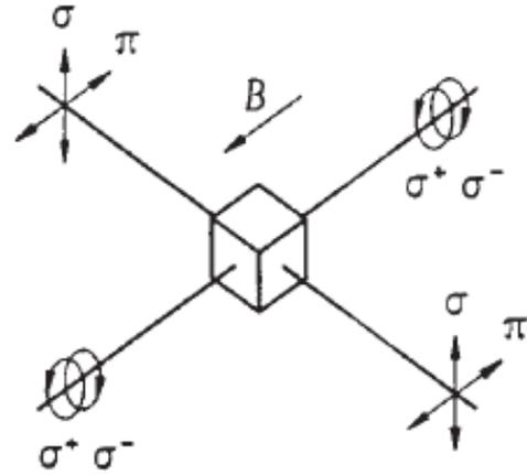
Figure 2: Longitudinal and transverse Zeeman effect.
